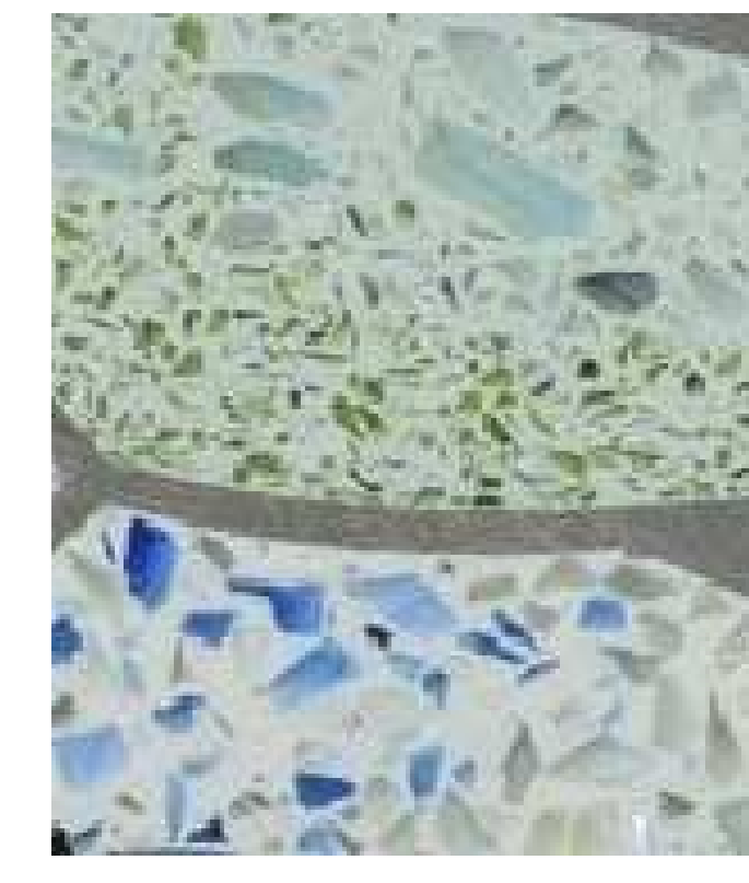
09 EXAMPLE OF AGG SCATTERING-RANDOM VARIATIONS TO AGGREGATE ACHIEVED BY SCATTERING LARGER AGG. AMONG REGULAR MATRIX JUST AFTER IT IS POURED, WHILE IT IS IN LIQUID STATE
