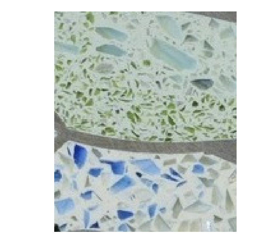
10 AI.114 EXAMPLE OF AGG SCATTERING-RANDOM VARIATIONS TO AGGREGATE ACHIEVED BY SCATTERING LARGER AGG. AMONG REGULAR MATRIX JUST AFTER IT IS POURED, WHILE IT IS IN LIQUID STATE
