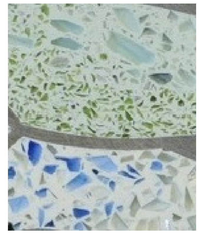
10 EXAMPLE OF AGG SCATTERING-RANDOM VARIATIONS TO AGGREGATE ACHIEVED BY SCATTERING LARGER AGG. AMONG REGULAR MATRIX JUST AFTER IT IS POURED, WHILE IT IS IN LIQUID STATE AI.114
